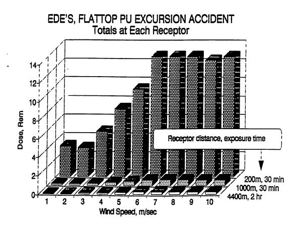
Figure 4-11: Receptor Total EDE's - FLATTOP Pu Excursion Accident
