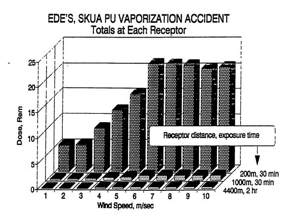
Figure 4-15: Receptor Total EDE's - SKUA Pu Vaporization Accident
