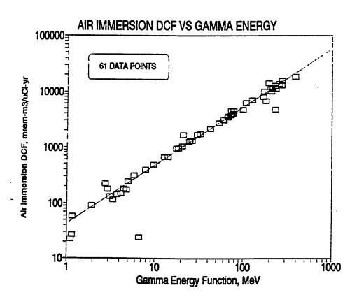
Figure 3-1: Air Immersion DCF vs Gamma Energy Function
