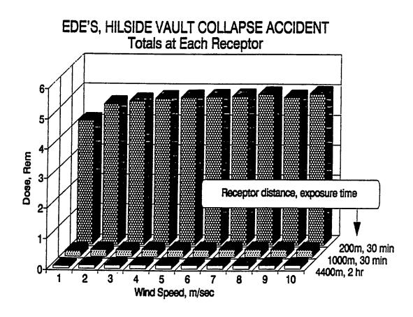
Figure 4-5: Receptor Total EDE's - Hillside Vault Collapse Accident
